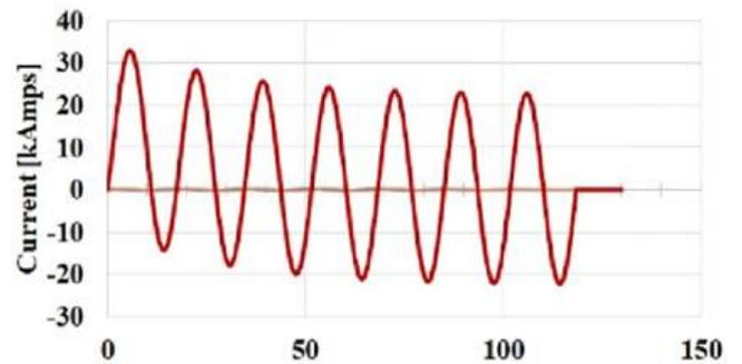
**7 cycles or more to clear the fault from de grid, adding incident energy, arc flash and arc blast which could be fatal for personnel.**
