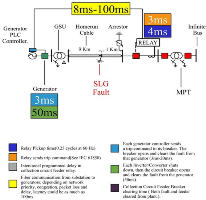
Fig. 6: Collection Circuit and Remote Transfer Trip.
