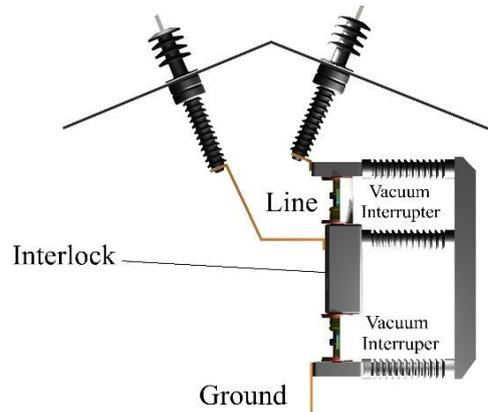
Fig. 2: Grounding Breaker (circuit breaker combined with a grounding switch) operates with one trip signal.
