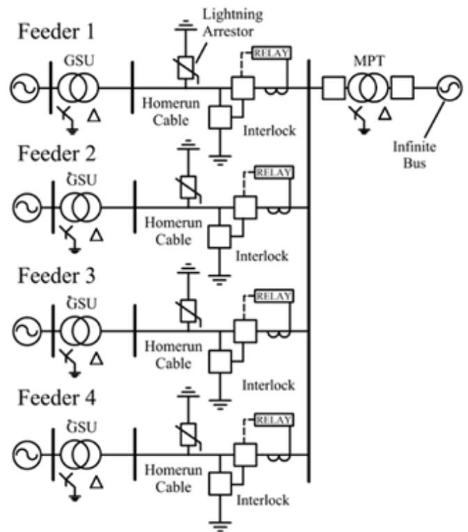
Fig. 3: WPP or SPP with Grounding Breaker Providing Protection at Each Feeder Circuit.
