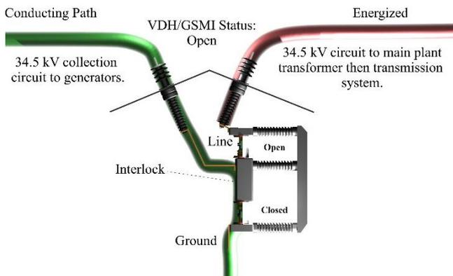
Fig. 5: Grounding Breaker in Open Status.
