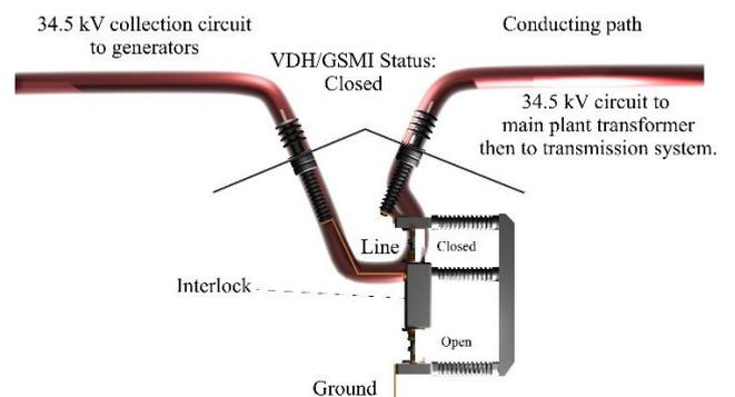
Fig. 4: Grounding Breaker in Closed Status.
