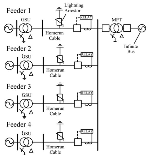
Fig. 1: WPP Single Line w/o Grounding breaker.
