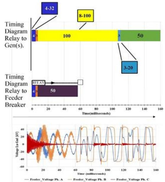
*Clearing the fault from the plant by opening the feeder breaker without a "programmed delay" and before the generators are off line results in less incident energy and the area of the arc blast boundary is much less; however, the TOV exceeds the prior duty curve of the lightning arrester and insulation coordination is lost, and that is bad.*
