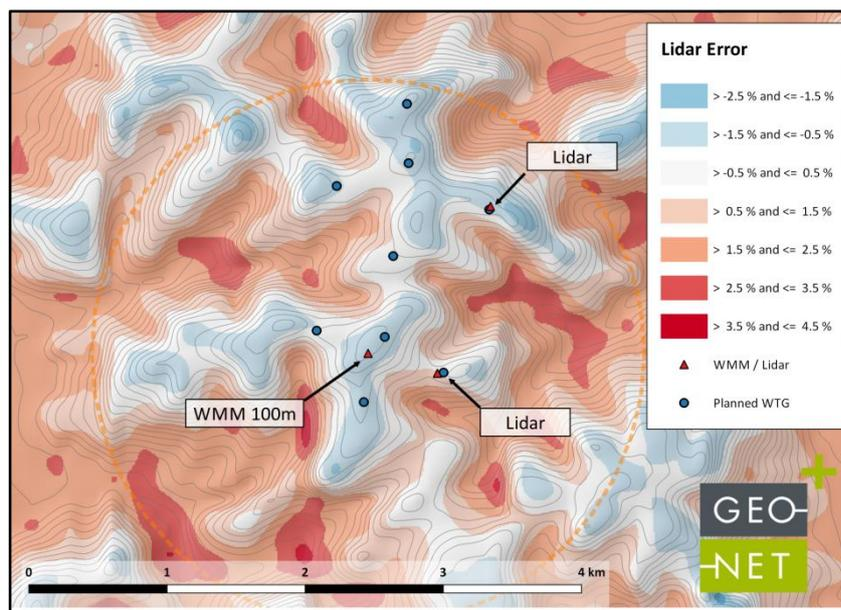
Figure 5 – Lidar error map.
