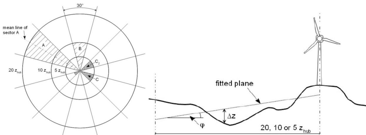
Figure 1 – IEC 61400-1 complexity test.
