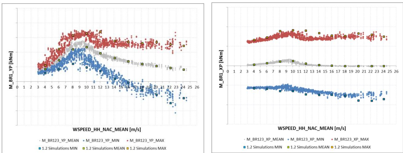
Figure 3: Statistical analysis result for blade root  $M_y$  and  $M_x$  bending moments.
