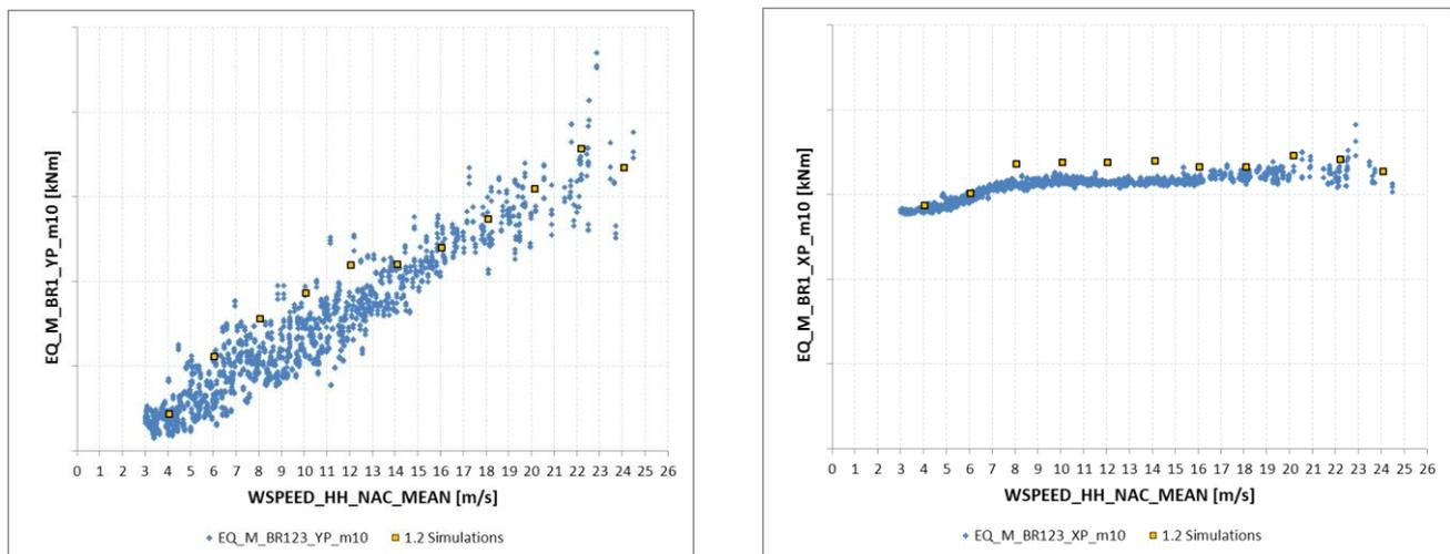
Figure 5: Equivalent loads comparison for blade root  $M_y$  and  $M_x$  bending moments  $m=10$ .
