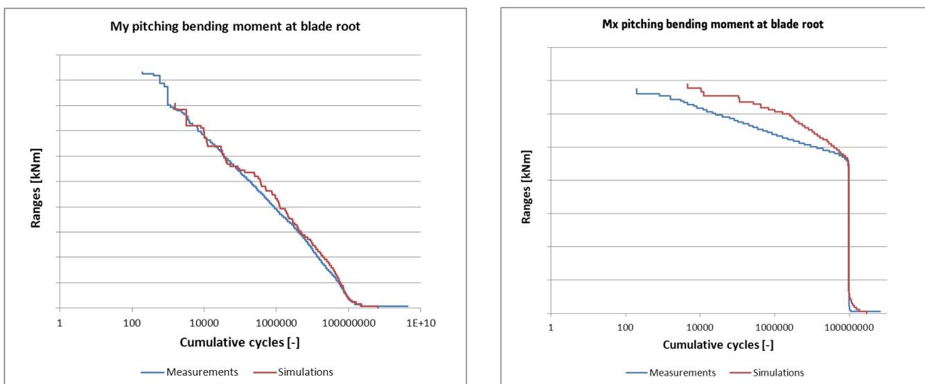
Figure 4: Rainflow cycle distribution comparison for blade root  $M_y$  and  $M_x$  bending moments.
