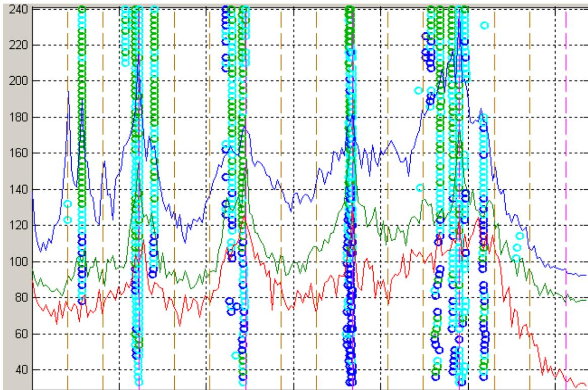
Figure 1: Example of stabilization diagram obtained as a result from OMA method.
